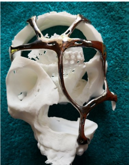
Figure (top): Centre for Rapid Prototyping and Manufacturing (CRPM) custom-designed titanium implant shown on a screen as part of planning activity between engineers and surgeons. Figure (below): The 3D printed titanium implant manufactured by CRPM and later successfully implanted. The implant is mounted on a plastic printed replica of the patient's bone structure.
