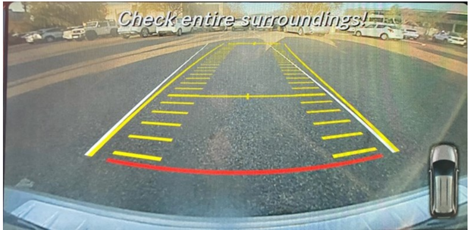
This image is from the control screen on a 2015 model car showing the reverse camera and the projected trajectory of the movement of the vehicle.
