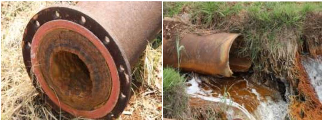
Pipes transporting **Acid Mine Drainage**. The photograph on the left shows a pipe with **precipitated** metals and the photograph on the right shows corrosion caused by **Acid Mine Drainage**.
