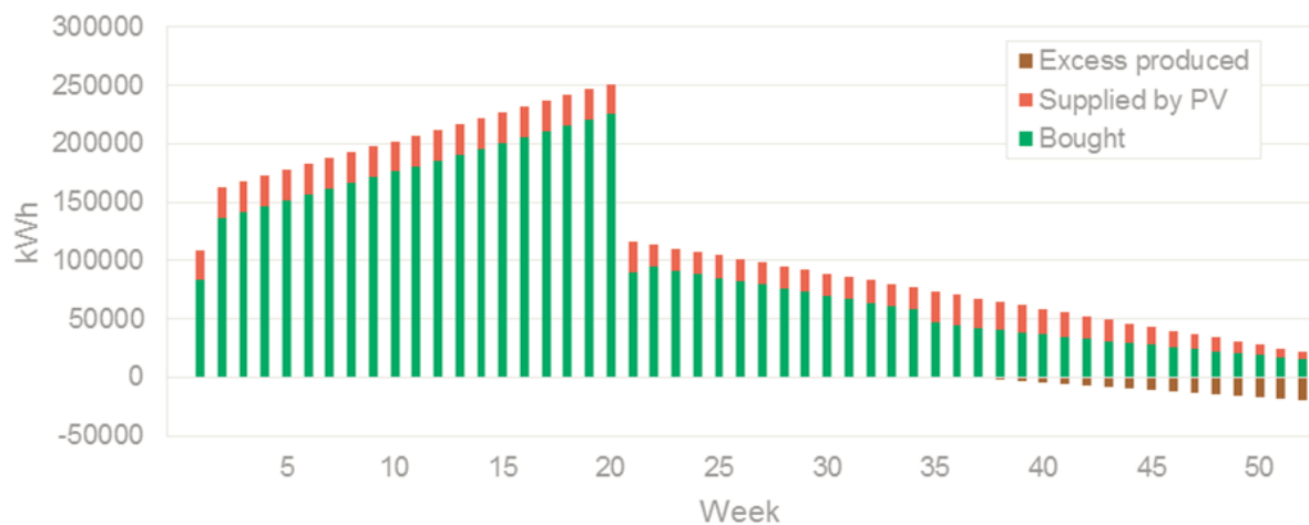
Figure 14: Electricity profile of a packhouse packing 1000 tonnes of apples a week with a 500 kW p solar PV system installed.
