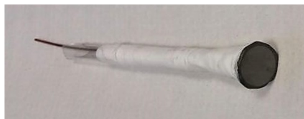
Figure 2: Genau Analytics' proprietary electrode to detect pollutants in water solutions
