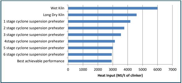
Figure 9: Thermal energy consumption by rotary kiln type<sup>13</sup>
